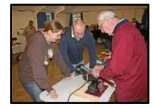
Trevor brought along his Robert Sorby ProEdge Sharpening system. This is a bit like a belt sander and can be used to effect the various grinds that woodturners use. Like other sharpening systems it uses various jigs to present the tool correctly to the belt. Trevor is seen here showing Tic Challis and Neil Robertson how it sharpens a skew chisel.
