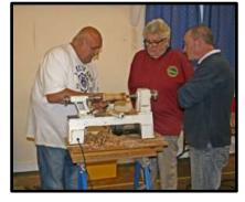
Maurice decided to use up some more of his stock of Ash and make a weed or dried grass pot. He first formed a spigot on the blank between centres then mounted it in the chuck. He then drilled a hole down the centre and began to shape the outside of the vase. In the photograph Sean Clifford is explaining some finer detail of technique.
